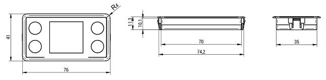
The LCD's mounting place surface (plastics or sheet metal) should not be thicker than 1,5 +/-0,1mm
